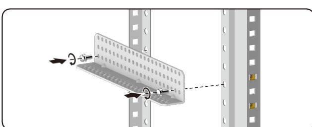
○ 安装设备到机柜 Install the router to the rack
