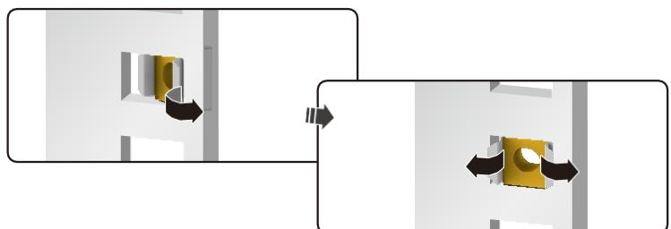
○ 在机柜立柱上安装两个托板 Install two support rails on cabinet
